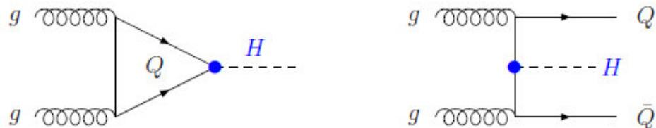
Higgs production in proton-proton accelerators by the fusion of two gluons
